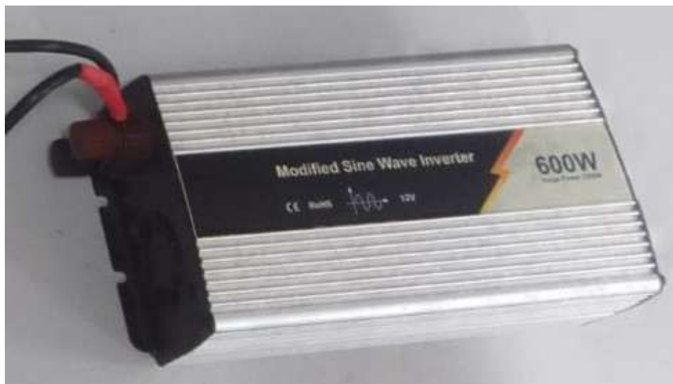
Figura 5.7 - Inversor Off Grid Jay Energy 12Vcc/127Vca (600W)
